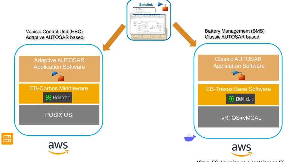
Virtual ECU running as an AMI on AWS Graviton
